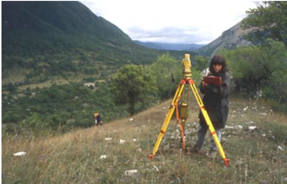
Total Station survey by Oliver Creighton (Exeter) and Luisa Dallai (Siena) on the height of Colle Sant'Ianni – the castle site of Rocca Intramonti lies in the background, above the distant ranging pole of Dr Creighton
